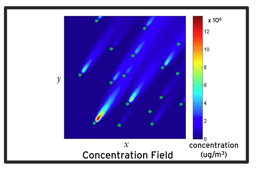
In reality, the concentration field is unknown. The sensing agent must infer the strengths of the fugitive emissions from concentration data collected along public roadways. This paradigm is referred to as inverse-dispersion. For the field site and concentration field above, the mobile sampling vehicle would obtain concentration measurements, such as those found below.
