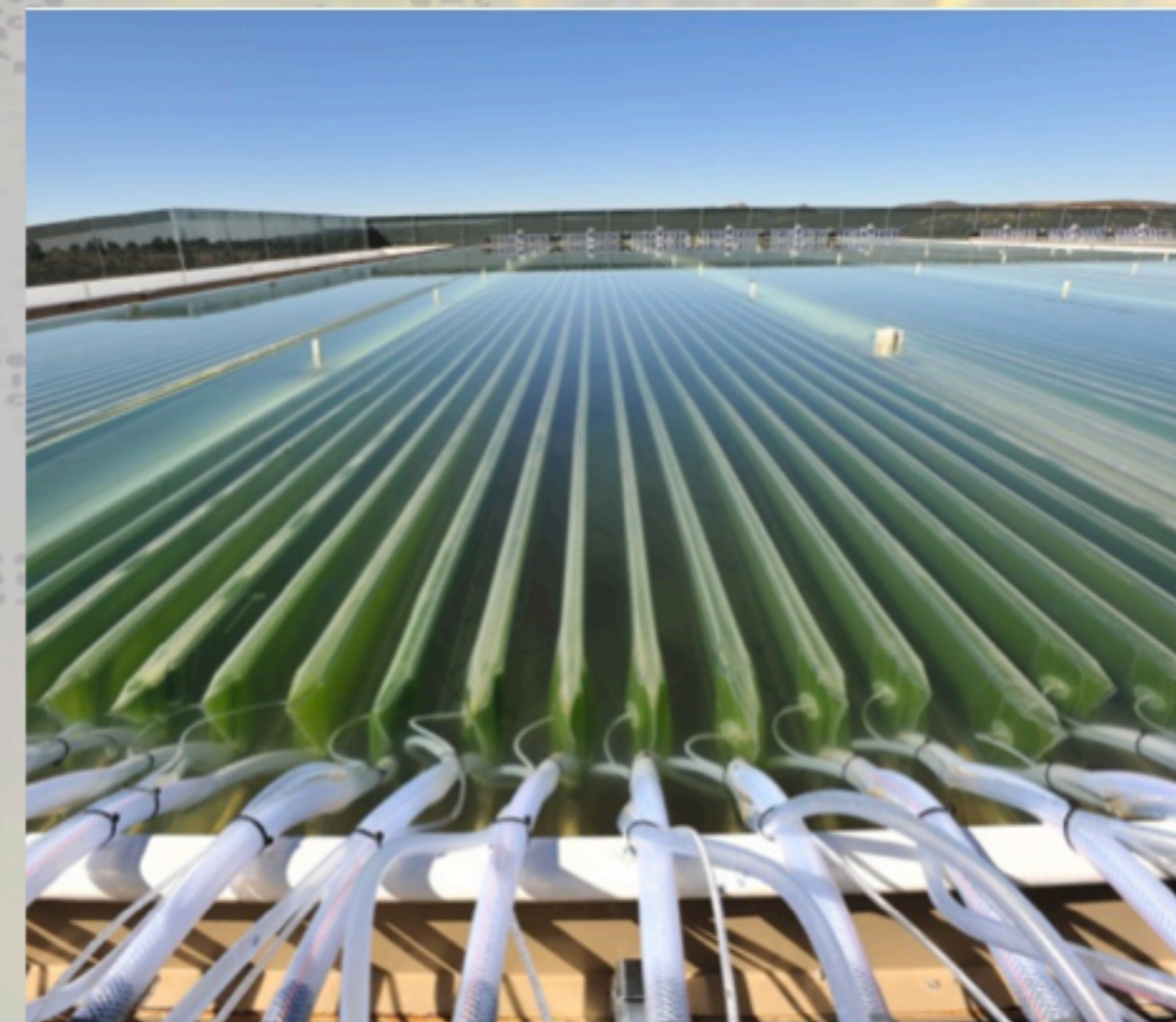
200L growth systems at Solix. A main goal is preventing biofilm buildup and invasion by bacteria and unwanted algae strains in these large-scale systems.
