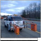
emits electromagnetic signals as it scans the surface along direction of vehicular travel The GPR signals reflect off of the rebar. Their amplitudes are decreased when corrosion is present in the concrete.
