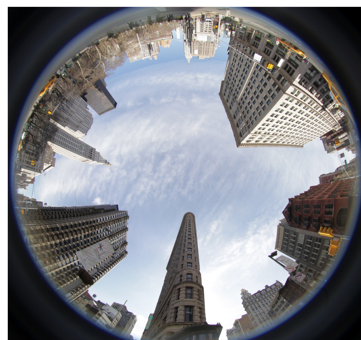
Figure 1— The sky view factor of the location shown above would be equal to the area of visible sky divided by the entire area of the circle. Structures such as buildings, trees and hills can reduce sky view factor and impact heat accumulation with in cities
